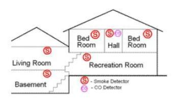
Mounting of Detectors on Walls/Ceiling:
